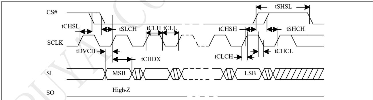
Figure 5-5 Output Timing
